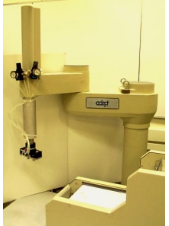
Fig. 14. Experimental workcell: the robot picks up parts from a convey belt using the parallel-jaw gripper.
